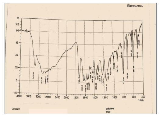
Figure 2. FT.IR spectrum of compound [6].
