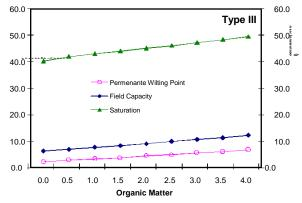
**Figure 3**. Change in soil water holding capacity (PWP, FC, saturation) under different dosage organic matter for soil Type I (Sand Clay Loam), Type II (Sand Loam) and Type III (Sand).
