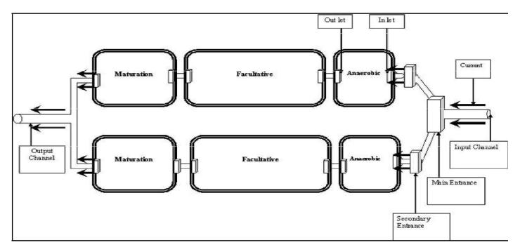
Figure 1. Pattern of soba stabilisation station ponds.
