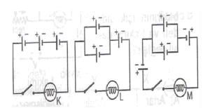
When the switches on, what is the relationships between the lights? (Cells and lamps are equivalent to each other)
