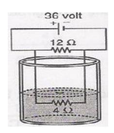
What will be the temperature of water after 5 min later? (cwater = 1 cal/g  $^{0}$ C , 1 cal 4 J, Heat transfer is only between conductor and water) I
