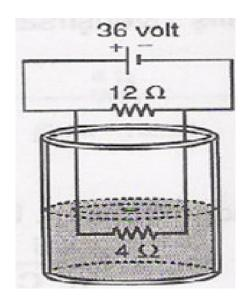
What will be the temperature of water after 5 minutes later? (c water = = 1 cal/g <sup>0</sup>C, 1 cal 4 joule, Heat transfer is only between conductor and water)
