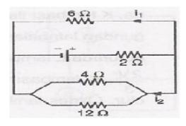
Given in the figure, What is the ratio of  $i_1 / i_2 =?$
