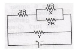
At the At the electrical circuits, current flows on the X resistor, is identical with Y resistor. According to the givens, what is the value of Y resistor?
