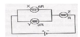
Given at the figure, what is the relationship between the light. (Lamps give off the same colour of lights).
