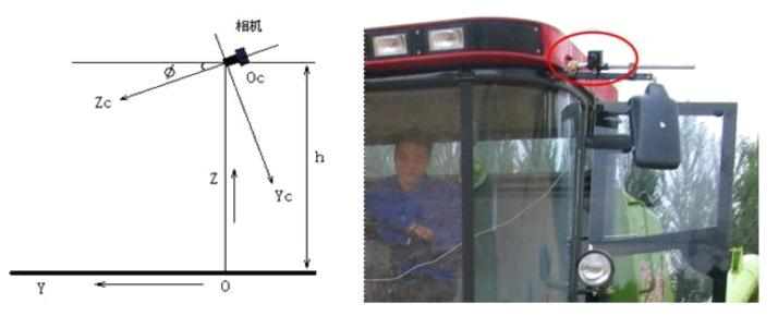
Figure 1. Camera installation and coordinate systems, the right are the combine harvester platform.
