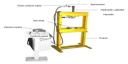
Figure 1. Hydraulic press setup.
