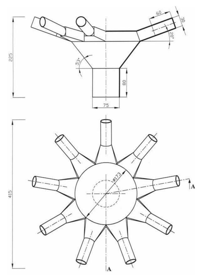
Figure 2b. Constructive properties of funnel distributor head.
