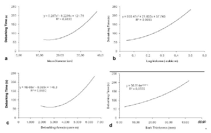
Figure 2. The relation between debarking time and average log diameter (a), log volume (b), debarking surface area (c), and bark thickness (d).
