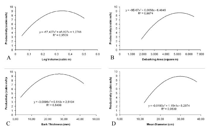
Figure 3. The relationship between work productivity and log volume (a), debarking surface area (b), bark thickness (c), and mean diameter (d).
