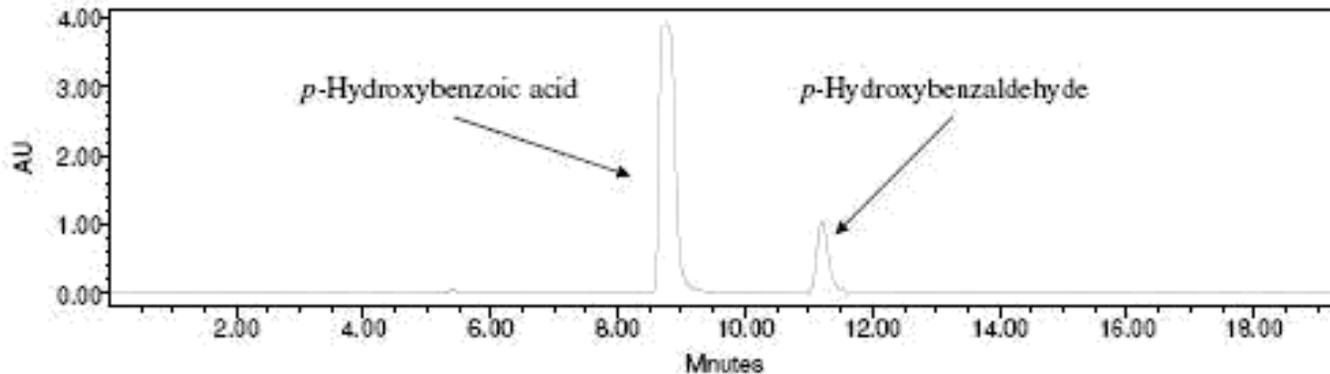
**Figure 6b.** HPLC Chromatogram representing the conversion of *p*-hydroxybenzoic acid to *p*-hydroxybenzaldehyde (reverse route) at 254 nm by mycelial cultures of *Schizophyllum* after 5<sup>th</sup> day of incubation.
