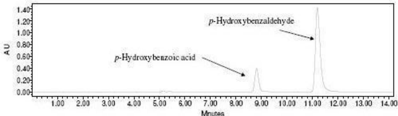
**Figure 6a.** HPLC Chromatogram showing the conversion of *p*-hydroxybenzaldehyde to *p*-hydroxybenzoic acid at 254 nm by mycelial cultures of *Schizophyllum* after 5<sup>th</sup> day of incubation.
