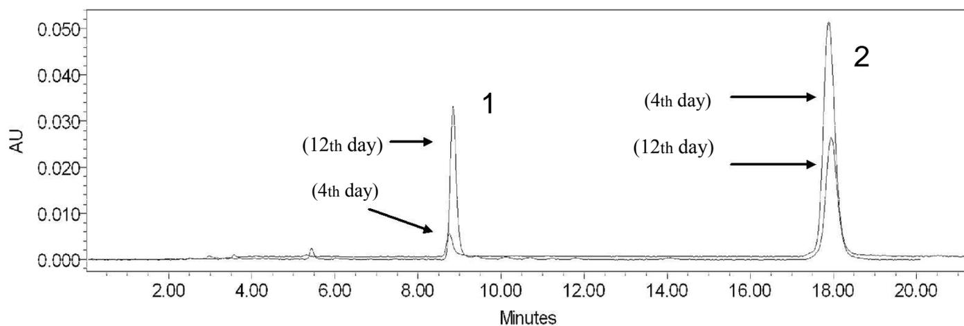
**Figure 3.** Overlay of HPLC chromatograms at 254 nm showing increase in the formation of *p*-hydroxybenzoic acid (1) and decrease in the concentration of *p*-coumaric acid (2) after 3<sup>rd</sup> and 11<sup>th</sup> day of incubation.
