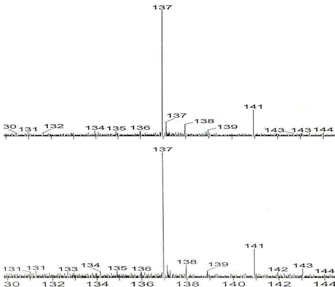
**Figure 4.** Mass Spectra of *p*-hydroxybenzoic acid produced from *p*-coumaric acid by *S. commune* (upper fragment) as compared to mass spectra of *p*-hydroxybenzoic acid standard (lower fragment). ESI-MS of HPLC purified samples was done in negative ion mode. X-axis shows mass to charge ratio, whereas Y-axis shows relative intensity.
