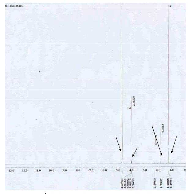
**Figure 1.** The 400 MHz <sup>1</sup>H NMR spectra of organic acids produced from fermented kitchen waste used as PHB substrate in this study. HLac- Lactic acid, HAc- Acetic acid.
