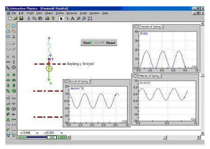
Figure 1. Harmonic motion simulation with interactive physics program.
